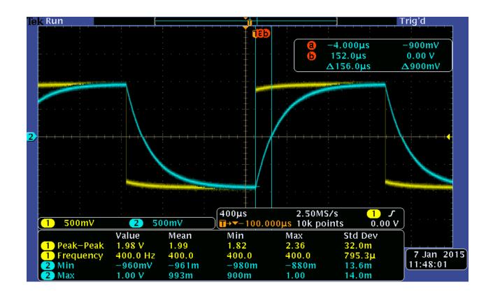
Make them **BIG**, input on channel 1, output on channel 2. Add useful on-screen measurements.
